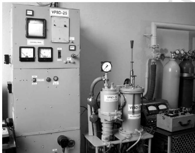
Fig. 1. The vacuum device VPBD-2S for boriding (boronizing) the metals, alloys and steels.
